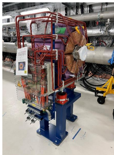
Positioning of a Sextupole module in line 2
