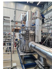
First of series testing of Super FRS local cryogenic components at STF: first P-Branch feed box plus transfer line, end box and triple arc jumper.
