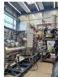
First of series testing of Super FRS local cryogenic components at STF: first P-Branch feed box plus transfer line, end box and triple arc jumper.
