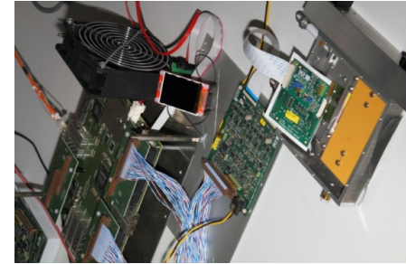
Customized FEE & DAQ, probe-testing of thin sensors
