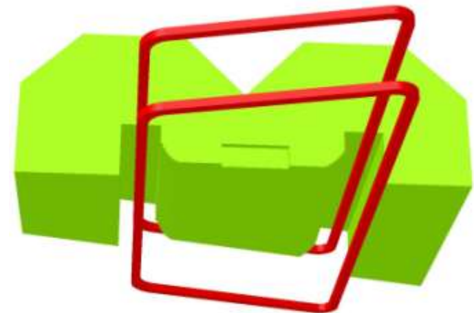
DIPOLE MAGNET FOR ENERGY BUNCHER - 2014
