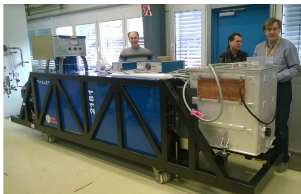
THALES Klystron by IN2P3/CNRS France 2.8 MW per pulse
