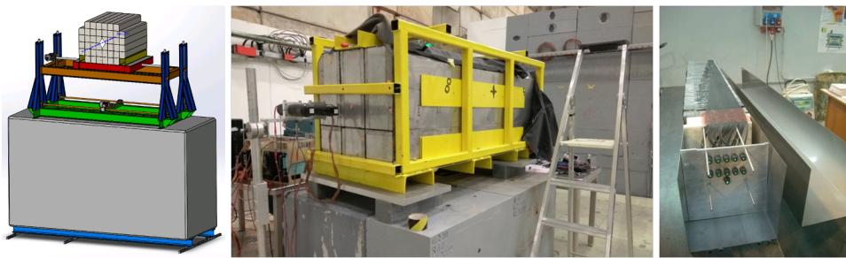
**Figure 3.14:** Design of the PSD with a support platform (left). PSD supermodule assembly (center). PSD module during installation (right) [59].
