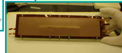
First GEM-TPC called HB1 detector (Helsinki Bratislava prototype 1)
