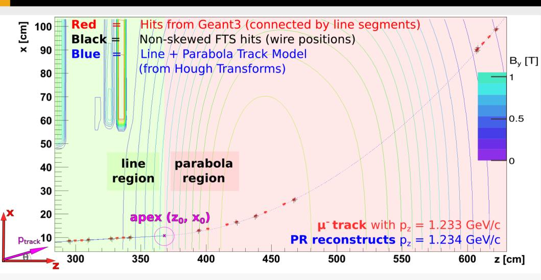
Simulations show that the tracks can be approximated by a line before, a parabola within, and a line behind the dipole field
