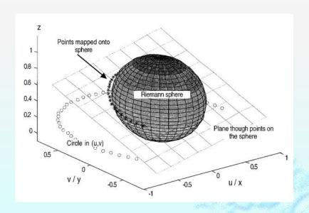
Particle tracks fitted on the Riemann sphere
