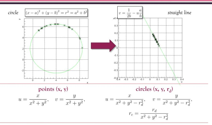
$\sim$  if the track does not stem from the IP  $\rightarrow$  make a translation onto a precise hit, such as an MVD, a SciTil or the center of the STT hit
