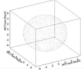
Tests were made with 1000  $\mu$  events generated over a sphere centered in the IP with radius = 6 cm - multiplicity = 2 - momentum = 1 GeV/c
