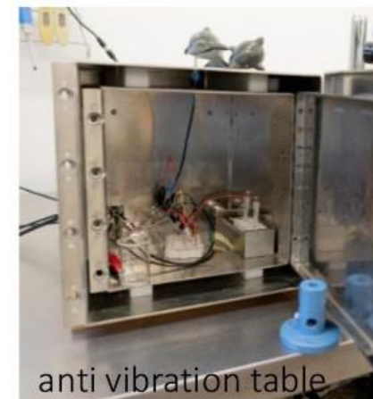
(a) double sided electromagnetic shield
