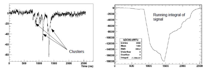
Figures from: Sam Dejong , Studies of Cluster Counting for use in SuperB Drift Chamber dE/dx measurements
