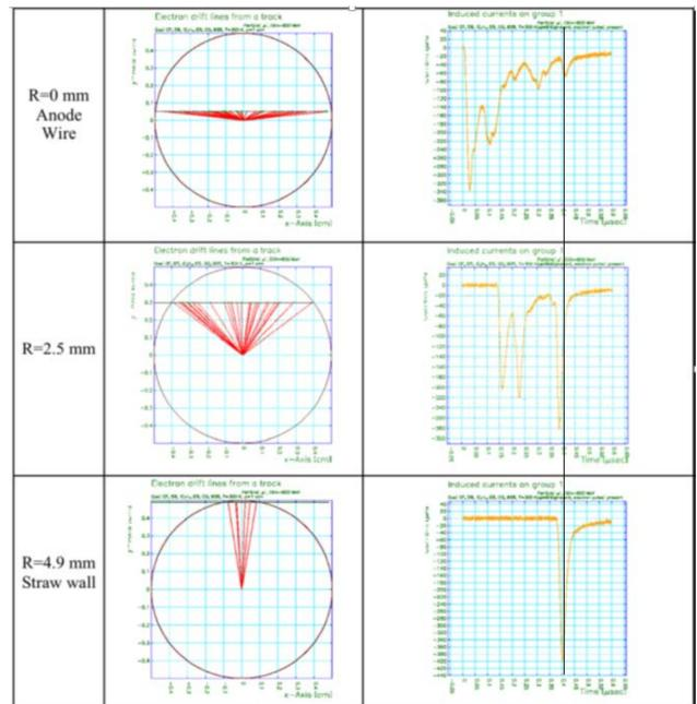
Figures from: Chapter Straw Tracker extract full doc, NA 62 Today we don't know what we see within 100.. 150 ns based on the single straw data. Possible multiple tracks and the amount of clusters belonging to the same track can not be detected.
