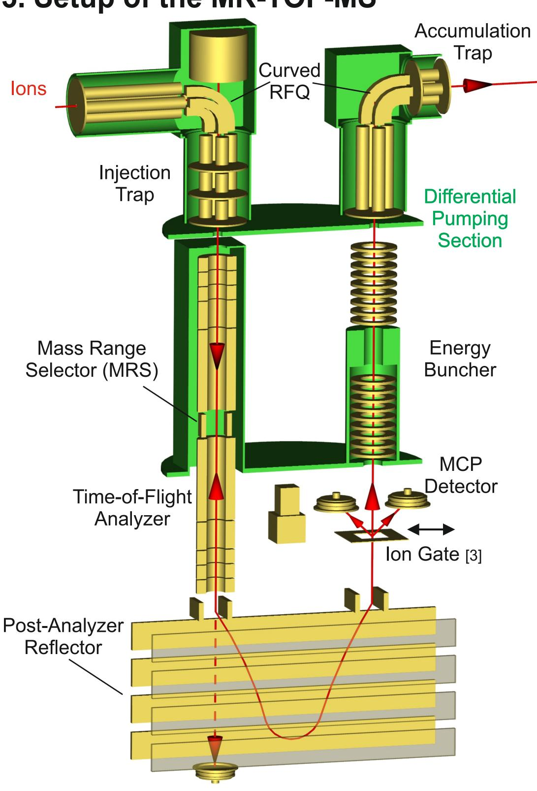
Schematic figure of the MR-TOF-MS system. The main functional elements are shown only. Overall height ~ 2 m, ion kinetic energy 750 eV
