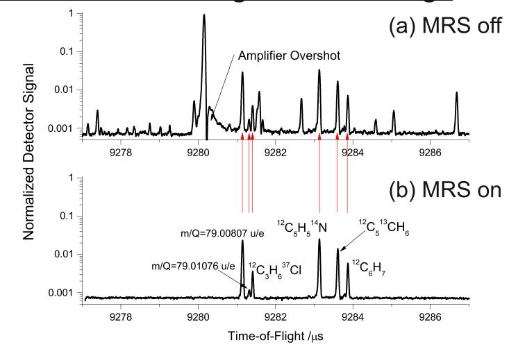
Time-of-flight spectra for mass 79 u of the mixture of benzene, pyridine and dichloropropane ionized by electron-impact ionization. (a) an identification of different masses is not possible because ions with different mass numbers have different number of turns. (b) Mass Range Selector (MRS) was set to exclusively transmit ions with mass 79 u. An unambiguous spectrum is obtained and the masses are measured and identified.
