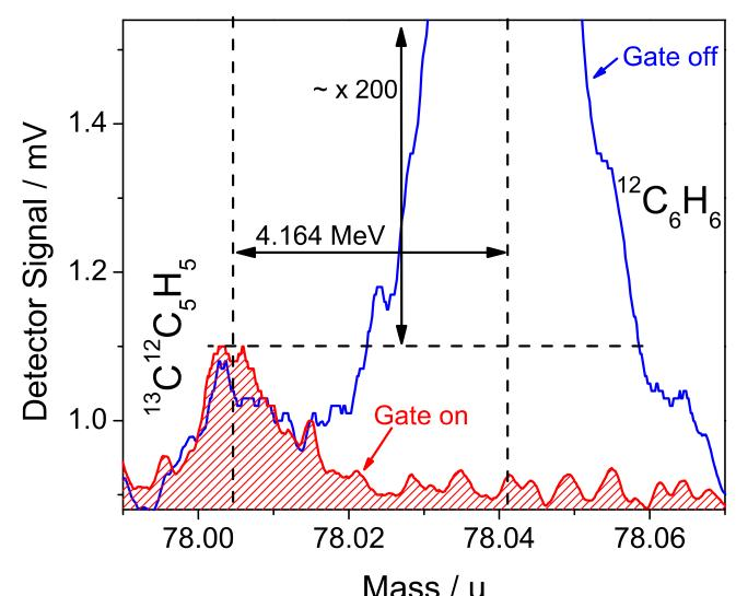
ratio (200). It can be clearly seen that the BNG deflects all <sup>12</sup>C<sub>6</sub>H<sub>6</sub> without disturbing the <sup>13</sup>C<sup>12</sup>C<sub>5</sub>H<sub>5</sub>. Note: The background is caused by electrical noise.
