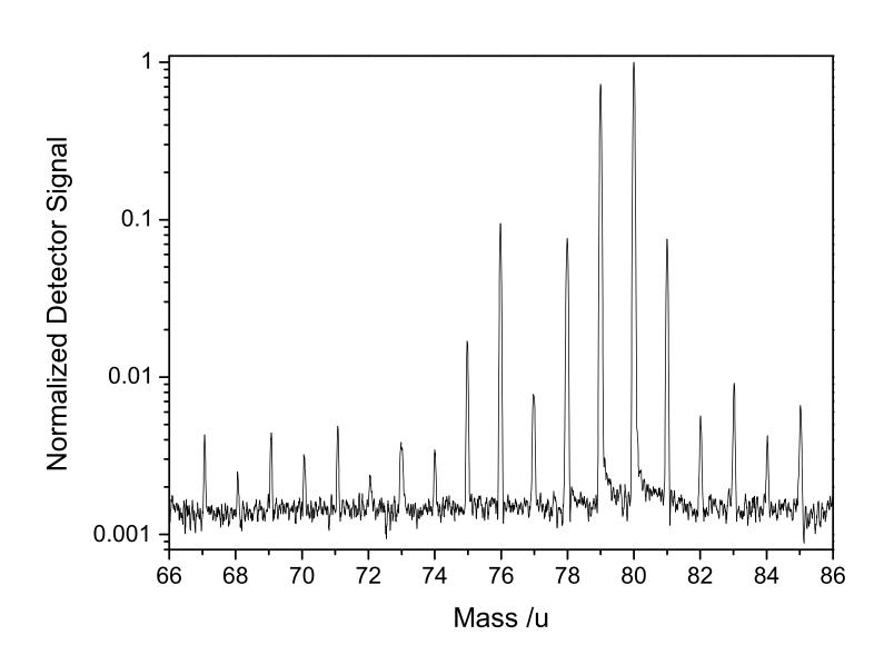
Measured broadband mass spectrum (pass-through mode) with logarithmic intensity scale of a mixture of benzene, pyridine and dichloropropane ionized by electron-impact ionization.
