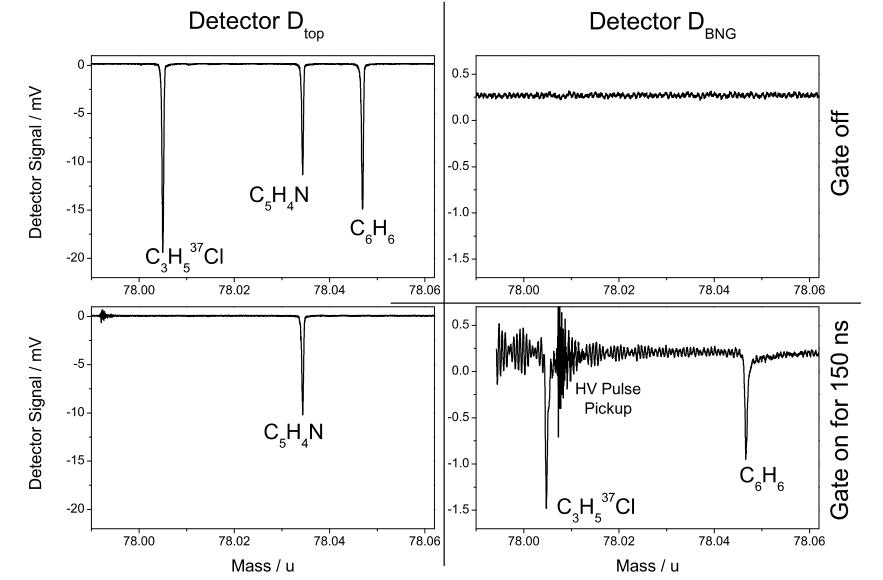
Measured mass spectra from a detector  $D_{top}$  (left hand side) and  $D_{BNG}$ (right hand side). The spectra in the upper panels are taken with the BNG off and in the lower panels the BNG is switched off only while the C<sub>5</sub>H<sub>4</sub>N ions pass through.
