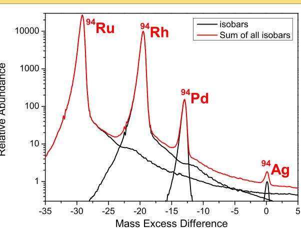
Expected mass spectrum of isobars at mass 94 u produced in the fusion-evaporation reaction <sup>58</sup>Ni(<sup>40</sup>Ca, p3n)<sup>94</sup>Ag. The relative abundances have been calculated with PACE4 and peak shapes measured with the MR-TOF-MS for <sup>133</sup>Cs have been used. It is apparent that a direct mass measurement of  $^{94}$ Ag ( $t_{1/2}$  = 34 ms) would be possible with the MR-TOF-MS
