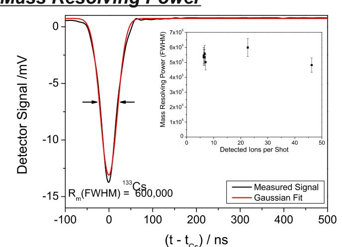
Mass resolving power of 600,000 (FWHM) (measurement time: 49 ms) is comparable to a 7 Tesla TOF-ICR-MS (measurement time: 1 s). The peak has a Gaussian-like shape even at this high resolving powers. This allows the separation of nearby peaks with largely different intensities. Inset: The measurement is independent of the number of detected ions, thus space charge effects do not influence the resolving power in this measurement.
