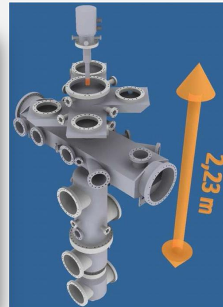
Layout of the new target inlet chamber design with the existing interaction chamber and target dump system for the ESR in Darmstadt.
