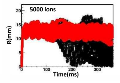
Increasing the number of ions makes the re-centering inefficient
