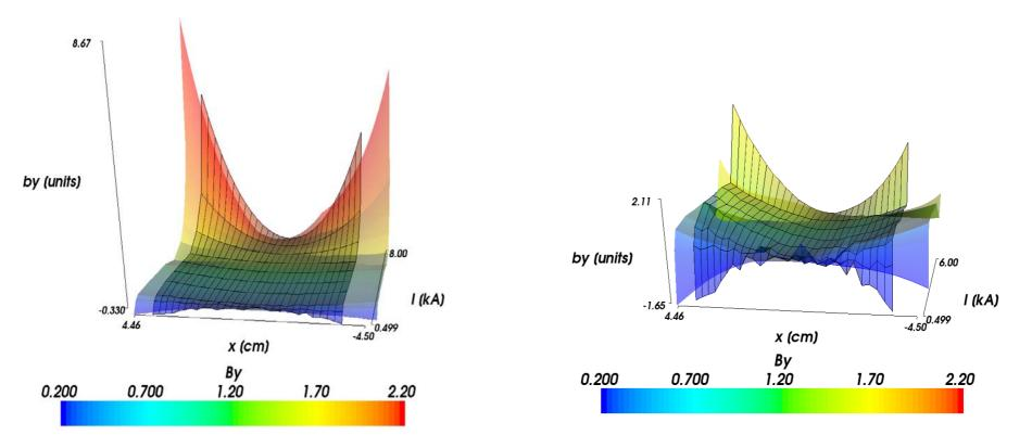
Field deviation in an area +/- 45 mm less than 2 units up to 1.75 T
