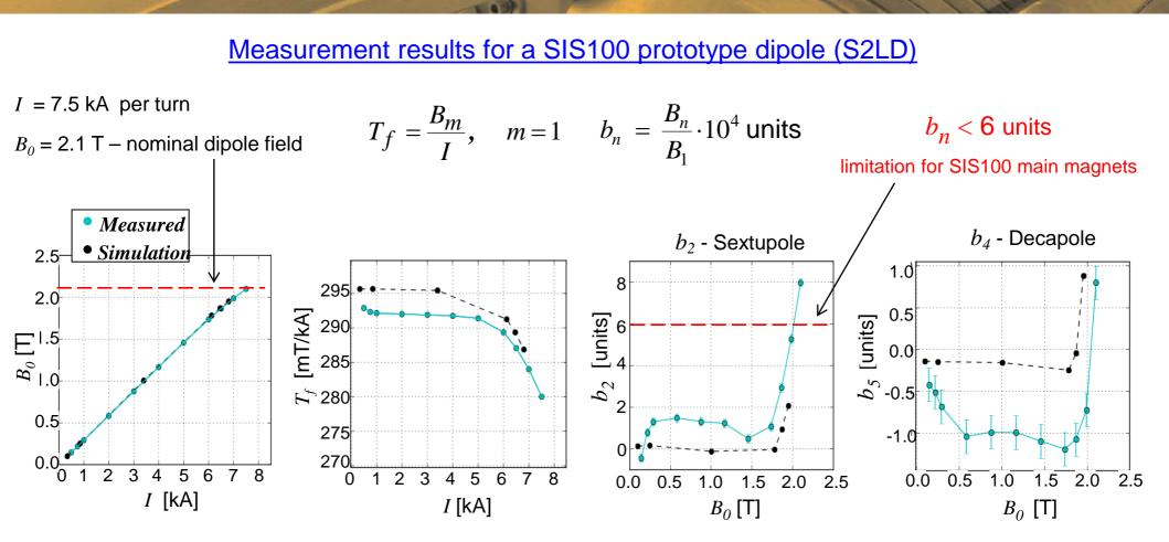
Simulation: 3D Model of the SIS100 prototype dipole (straight magnet with a double layer coil) Vector Fields Opera<sup>®</sup>, Measuring: rotating coil probe inside an anticryostat,
