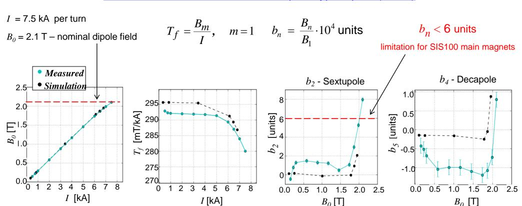
Simulation: 3D Model of the SIS100 prototype dipole (straight magnet with a double layer coil) Vector Fields Opera<sup>®</sup>, Measuring: rotating coil probe inside an anticryostat,
