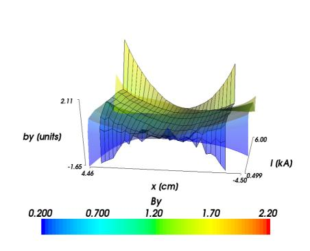
Field deviation in an area +/- 45 mm less than 2 units up to 1.75 T
