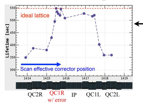
Position dependence of the skew corrector coil is stronger than that of normal.
