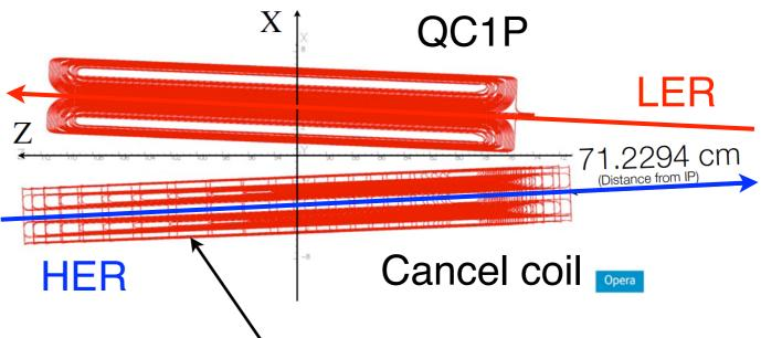
Cancel coil consists of  $b_3$ ,  $b_4$ ,  $b_5$ ,  $b_6$  coils ( $b_1$  and  $b_2$  are involved in the optics design.)
