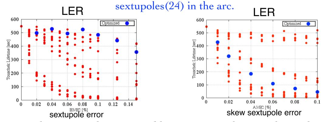
Sextupole error can be recovered by using normal sextupoles(in the arc), however, skew sextupoles error can not be corrected for enough level.
