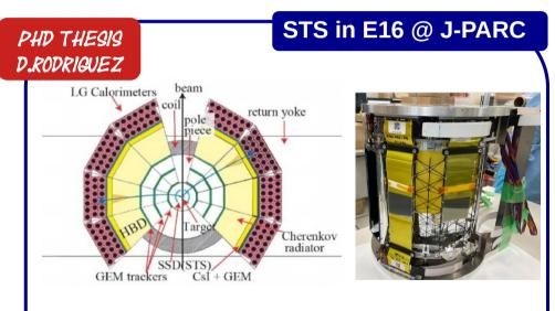
10 pre-series STS modules were built, assembled and tested at GSI and are installed as innermost tracking detector of the E16 experiment at J-PARC.
