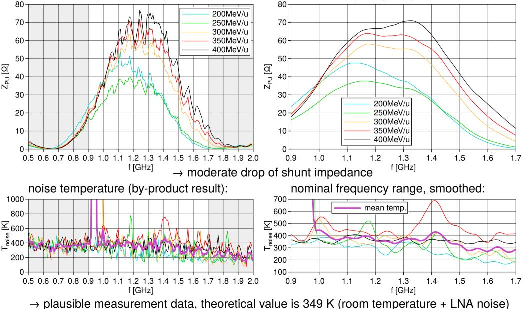
→ plausible measurement data, theoretical value is 349 K (room temperature + LNA noise the peak at 934 MHz is probably an irradiation from GSM-900 net
