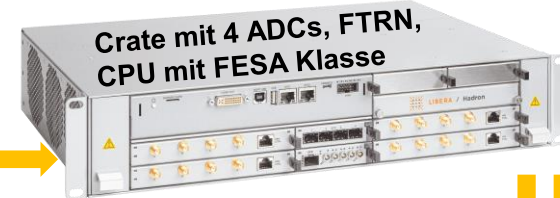
3) DAQ system: 2x Libera Hadron HEBT (250 MSa/s, 16 nom./12 eff. bits)
