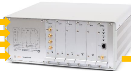
2) Front-end: HPA110 Verstärker 50 Ohm, BW = 55 MHz, Gain = [-50,+60] dB
