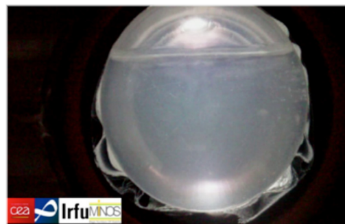
Front view of the target during the filling phase (the top part of the target cell is not filled yet).
