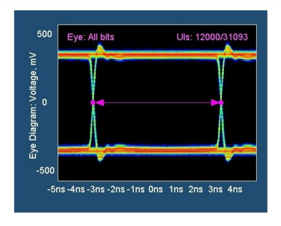
Analysis for the total jitter on the daisy chain lines connecting Topix clock and control signals at 156 Mb/s, for the short path to the first chip (on the left), and for the long path to the last chip (on the right).
