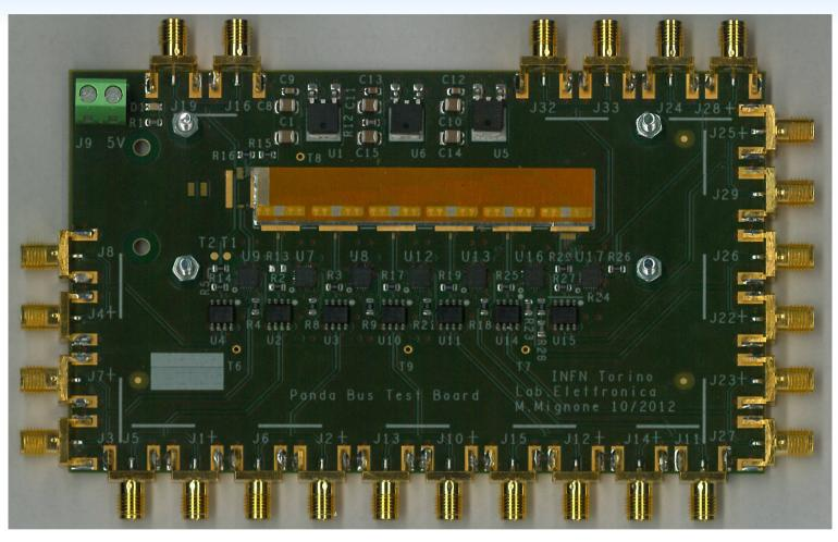
The test board contains LVDS/SLVS transceivers and buffers. These first tests were done using the Agilent N5980A BERT (Bit Error Rate Tester) equipment.
