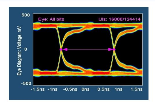
Analysis for the total jitter on the direct lines for Topix serial data output with the transceivers on the test board at 156 Mb/s (on the left), or without the transceivers on the test board at 622 Mb/s (on the right).
