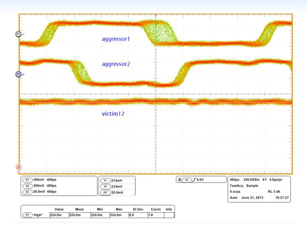
Analysis for the cross talk on the direct lines connected to the Topix serial output: in this case the victim line driven to a high state is subjected to both the aggressor1 and aggressor2.
