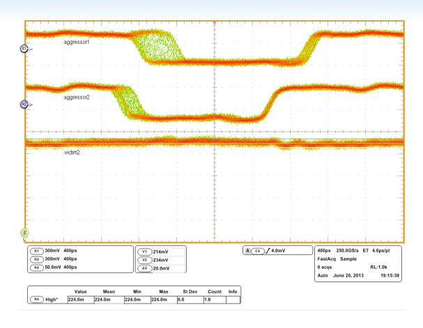
Analysis for the cross talk on the direct lines connected to the Topix serial output: in this case the victim line driven to a high state is simply subjected to the aggressor2.
