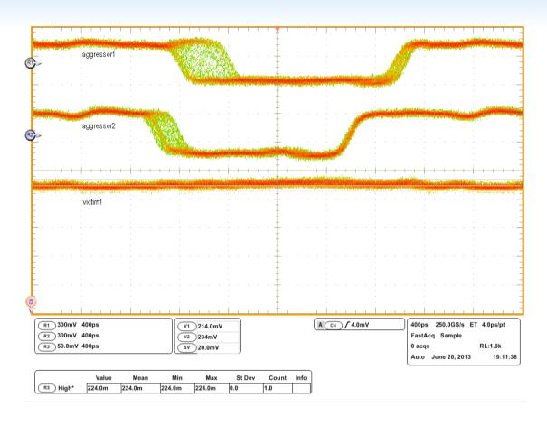
Analysis for the cross talk on the direct lines connected to the Topix serial output: in this case the victim line driven to a high state is simply subjected to the aggressor1.
