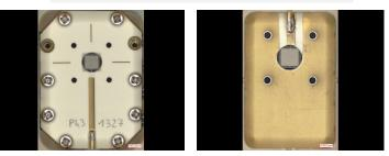
4x4mm<sup>2</sup> size ~480um thickness, Al electrodes
