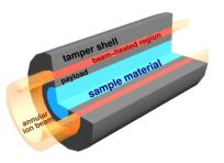
ring-shaped beam implodes a heavy tamper shell, low-entropy compression of hydrogen
