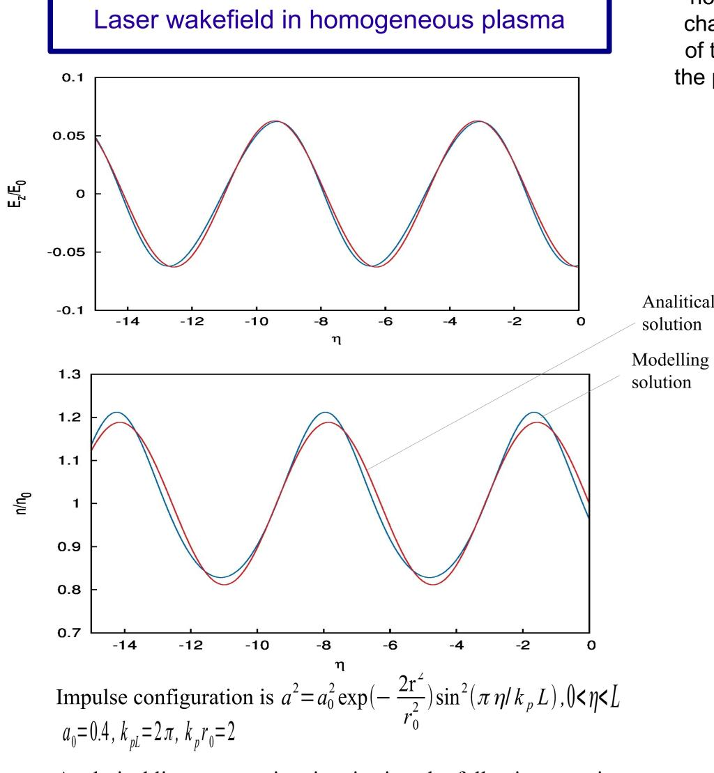
The structure of plasma waves excited by intense laser pulses or beams of charged particles is
