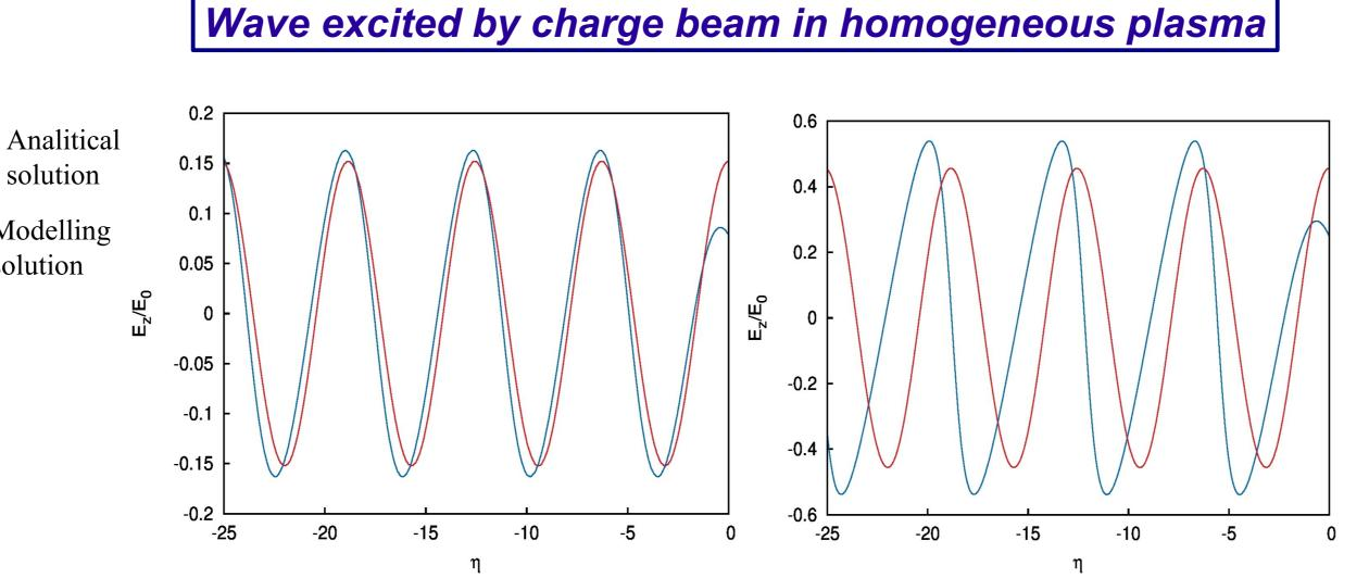
Wave excited by ion beams. Beams shape is given by :  $\rho(r, \eta) = \{ \begin{array}{l} n_b \exp(-\eta^2 / (k_p L)^2) & \text{if } r < r_0 \\ 0 & \text{if } r > r_0 \end{array} \right.$
