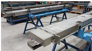
Actual picture (last Friday): half yokes are produced (laser welded by sub-contractor in Rostock)
