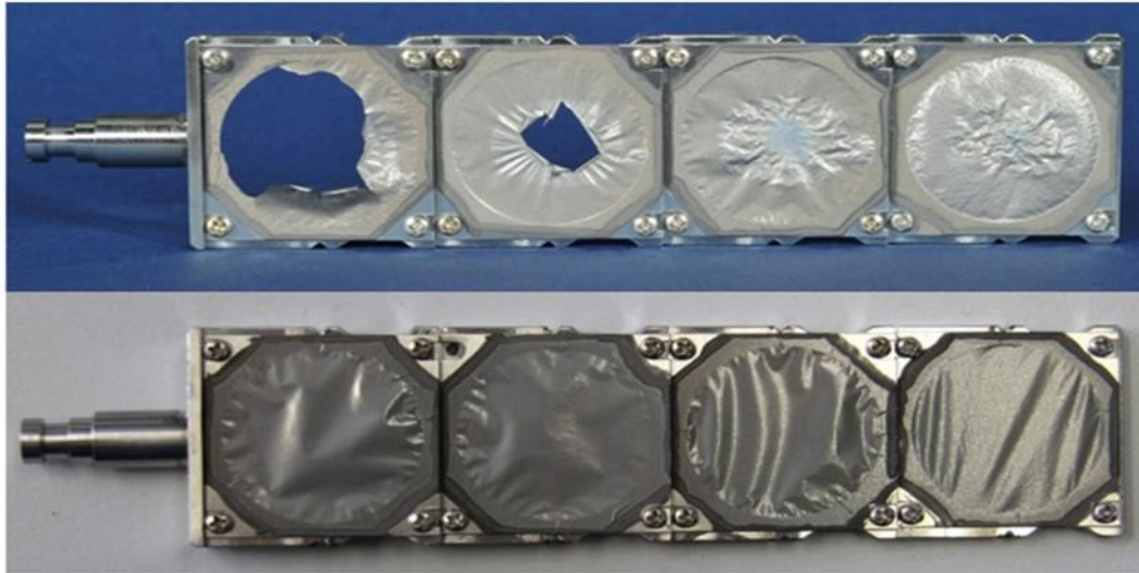
Carbon foil stripper before (bottom) and after (top) high current operation.
