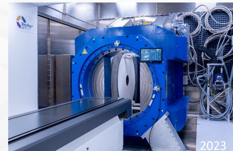
0.5 T in-beam MRI at PBS beamline:
