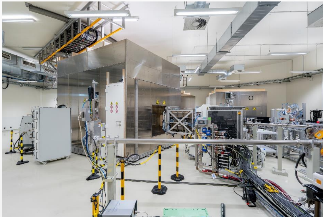
Back side of RF shielding attached to PBS Beamline
