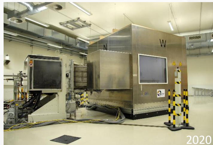
0.32 T in-beam MRI at PBS beamline:
