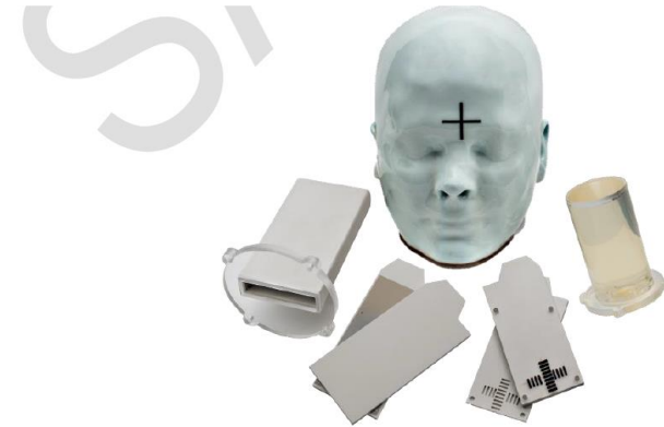
Figure 1: The RTsafe Prime phantom used in the audit, along with the specially designed inserts to accommodate Gafchromic EBT film, OSL and polymer gel dosimeters.
