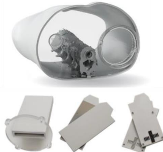
Figure 1: The RTsafe Prime phantom used in the audit, along with the specially designed inserts to accommodate Gafchromic EBT film, OSL and polymer gel dosimeters.
