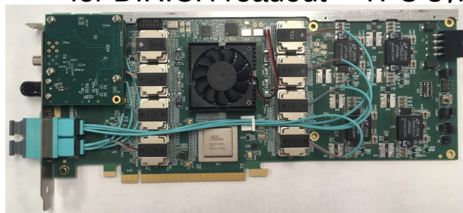
Figure 1: The FLX-712 card with fibres assembled.
