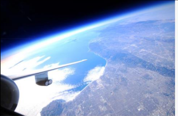
Figure 1 - Two round, large-area cosmic dust collectors deployed beneath the wing of a NASA ER-2 aircraft in flight.
