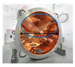
10 half-size drift tubes and 177 full-size drift tubes including two stems each
