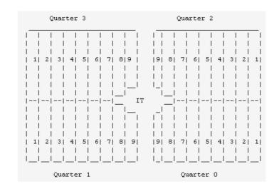
At the central region: (LHCb)  $0.32 \times 30$ MHz = 9.5 MHz/straw (CBM\*)  $\sim 0.086 \times 10$  MHz = 0.86 MHz/straw
