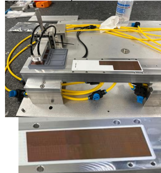
2 rows of 3 ALPIDE chips aligned on the jig
