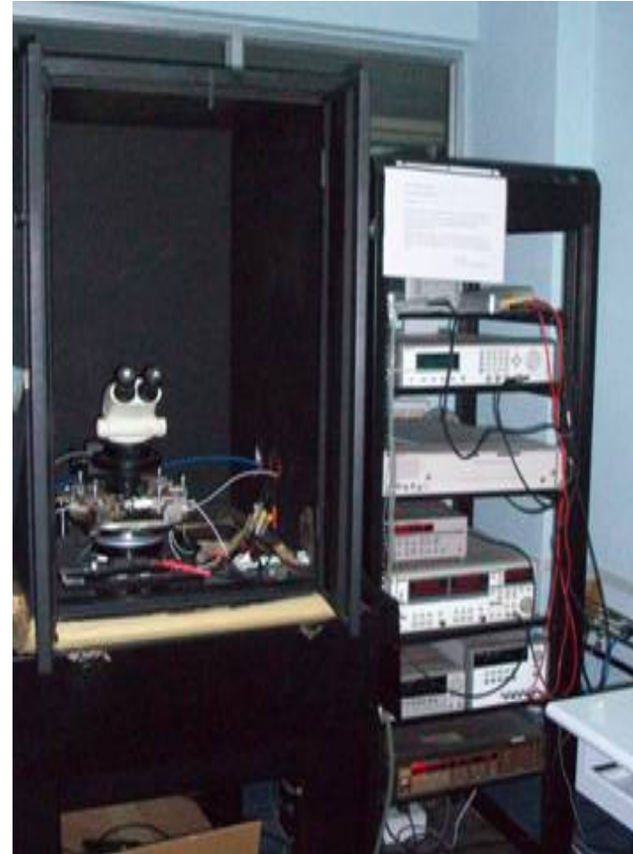
Vega: I-V Characterization setup
