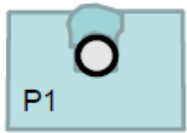
P1 Welding tube inside
