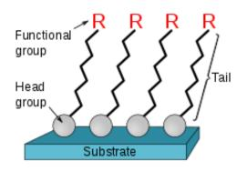
The use of selfassembled monolayers (SAMs) to functionalize surfaces of alpha detectors is currently under investigation
