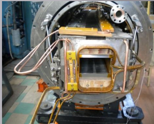
Dipole magnet in cryostat
