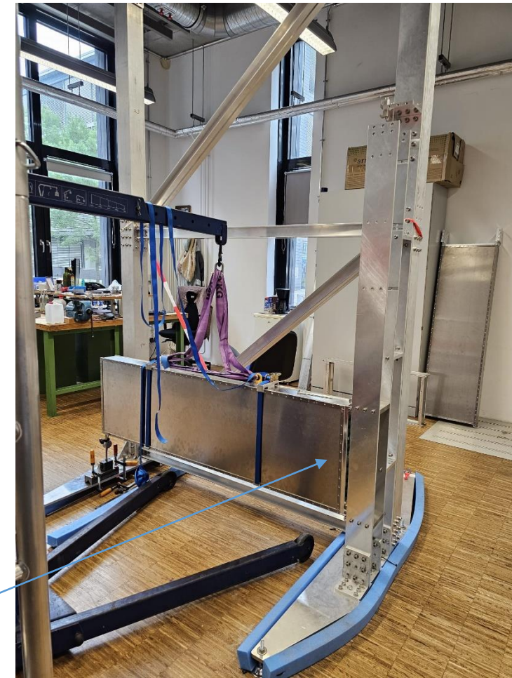
Stability test in mockup frame
