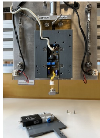
wire tension measurement: rework to reach edges in chamber and activated pitch evaluation
