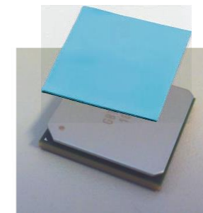
GBTX ASIC with Cooling Interface and Thermal Pad
