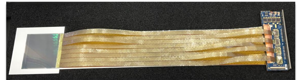
STS module before the shielding layers are soldered
