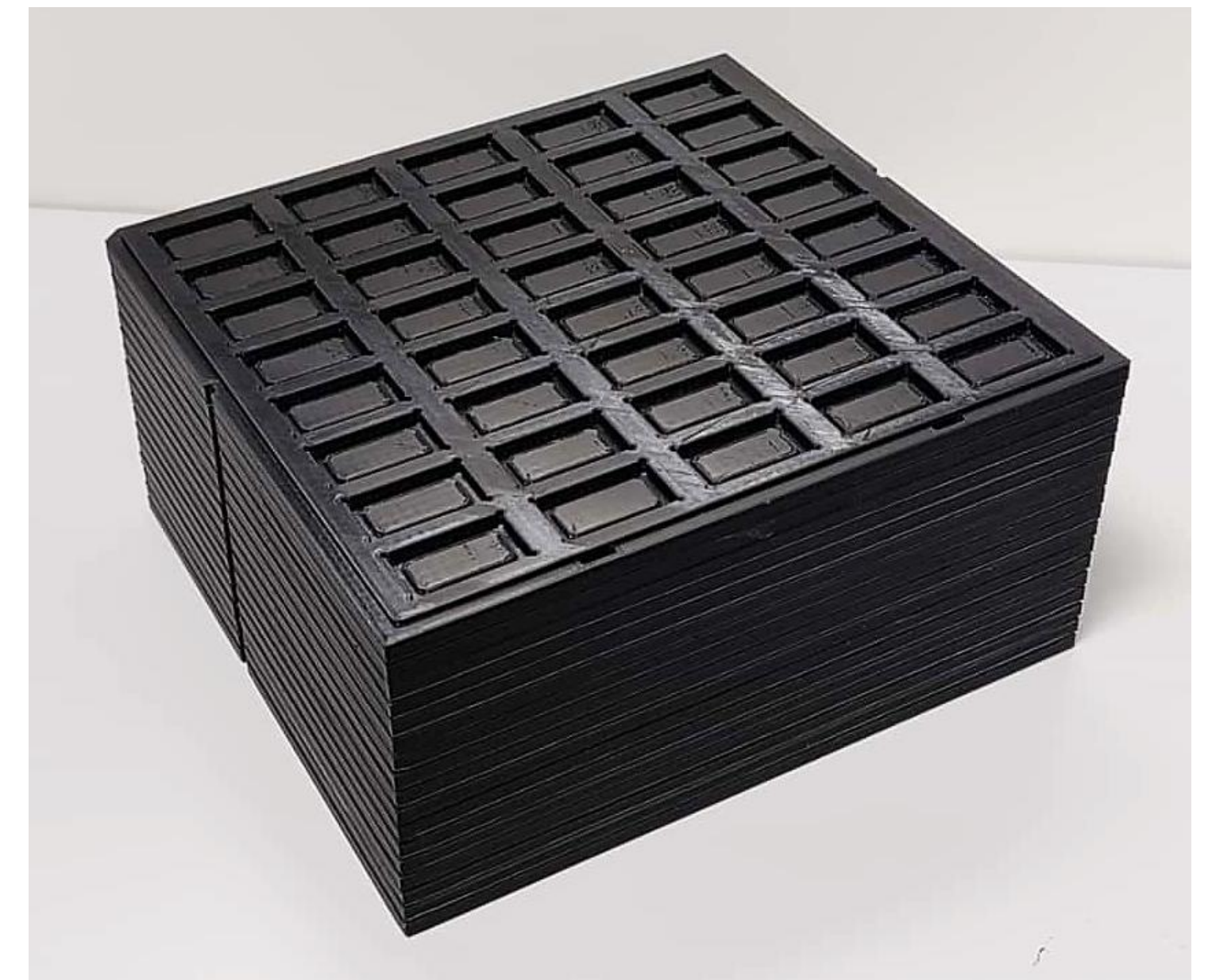
Dedicated transport boxes for 50 \mu\text{m} sensors (ALPIDE inspired)
