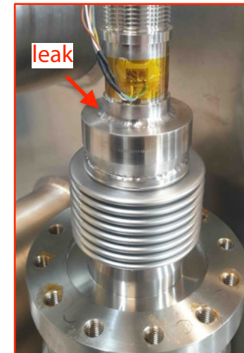
After repair, leak test
