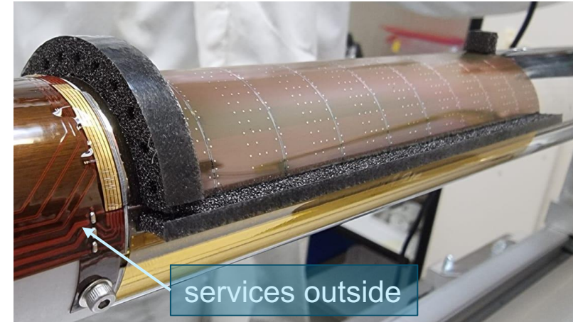
thin (<math><50\mu\text{m}</math> CMOS can be curled)
