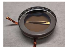
43 mm device with no MCPs – test of cooling and quantum efficiency
