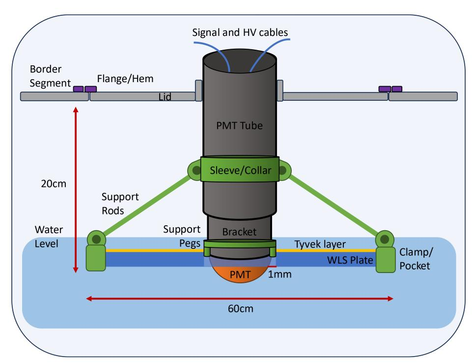
• Reflective edges guide photons toward the PMT photocathode.
