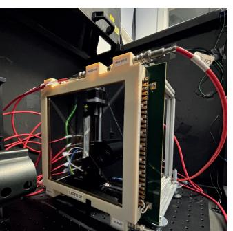
Lab measurements of the LAPPD with the RICH test beam readout chain were conducted using a custom picosecond 405 nm Pilas laser (timing jitter < 2ps).
