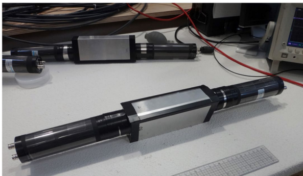
A threshold-type Cherenkov counter at J-PARC.
