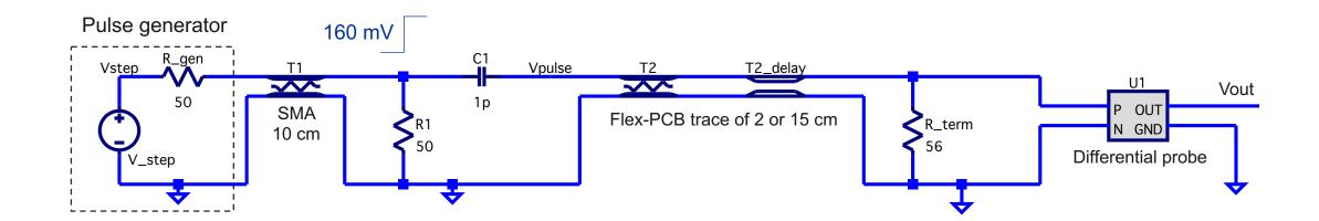
The main concern for the flex-PCB is the **impact of high-density**, **centimetre-long traces on signal integrity and time resolution**. The two test-pulse injection circuits were used to address this.
