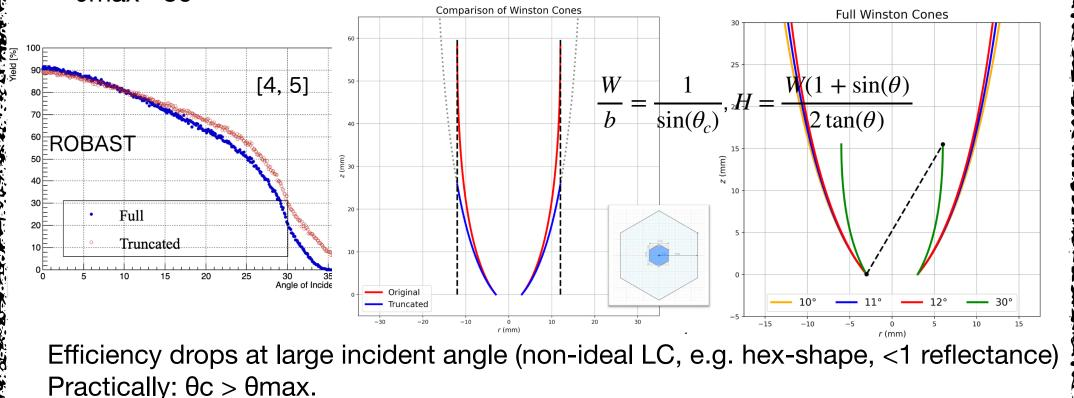
Larger  $\theta$ max  $\rightarrow$  smaller entrance size = more channels Optimising by truncating LC height Baseline design: Hexagonal Fallback option: Winston cone Conical shape, circular cross section
